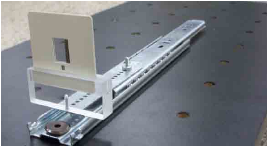
Razor blade in a slide holder to be placed in acrylic support (LABEL D1) and mounted on sliding rail (LABEL D2).
